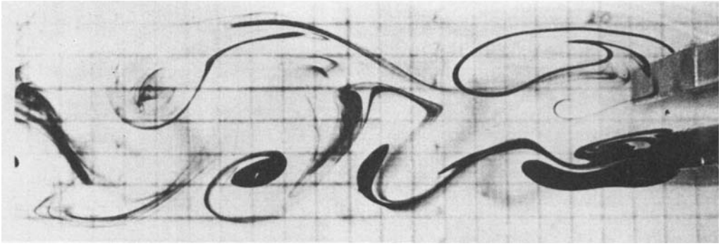
FIGURE 12. Second harmonic mode of vortex shedding from two flat plates. Dye visualization in the water channel, flow is from right to left, Re = 200 , g^* = 1.0 . In this case the gap flow is deflected to the lower side of the wake.
